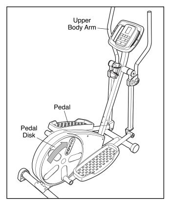
To dismount the elliptical exerciser, allow the pedals to come to a complete stop. **CAUTION: The elliptical exerciser does not have a freewheel; the pedals will continue to move until the flywheel stops.** When the pedals are stationary, step off the highest pedal first. Then, step off the lowest pedal.
